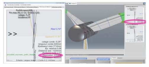
The Reynolds number for this item is around 370,000 and the naca 1408 profile gives us a maximum lift/drag ratio of 50. Looking for in our database of profiles, more efficient profile to this Reynolds number:
