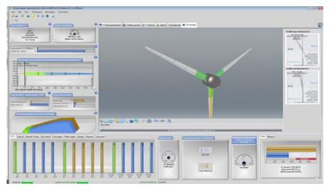
Our wind turbine and blade's twist is rebuilt, Results are given in the Output pane at the bottom of the screen. The shaft power is 523 Wattsand our rotor's efficiency is 0.443. Heliciel twisted blades, profiles see the fluid with an optimal incidence angle, generating an otptimal lift drag ratio (according to induced velocities). Our propeller in its current geometry and the current operating point is at its optimal twisting, all other settings in twists give inferior performance...
