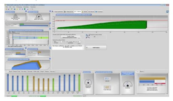
We get optimum speed 122 rpmThis speed decrease is Conform to phenomenon described above, but the surprise is the efficiency reaching the Betz limit therefore the theoretical optimum. It is theoretically impossible to make a wind turbine with better performance. The only drawback is that 13 blades, it's a bit expensive to manufacture...but how to explain this increase of efficiency?
