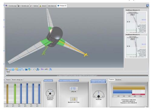
We obtain optimal performance slightly above the Betz limit, which is theoretically impossible! (no panic it exceeds 0.9 watts for 688 watts, this is just a calculation imprecision ). We could increase the number of elements (tab " optionals tools") to increase the accuracy (made the test with 10 items and you'll be 675 watts)
